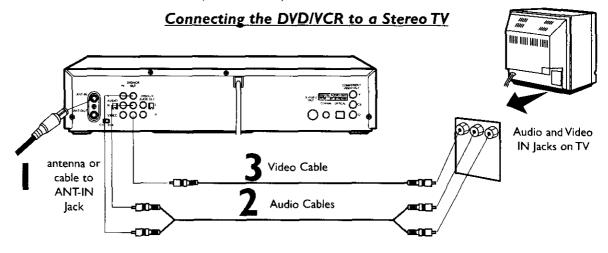
Connect the antenna or cable to the ANT-IN (Antenna in) jack of your DVD/VCR.
